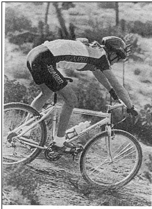
Figure M10.4.3.2.3.3 (b) Photograph of the Stump-jumper M2 bicycle, the frame is made from Duralcan ® 6061 Al-10wt% alumina
