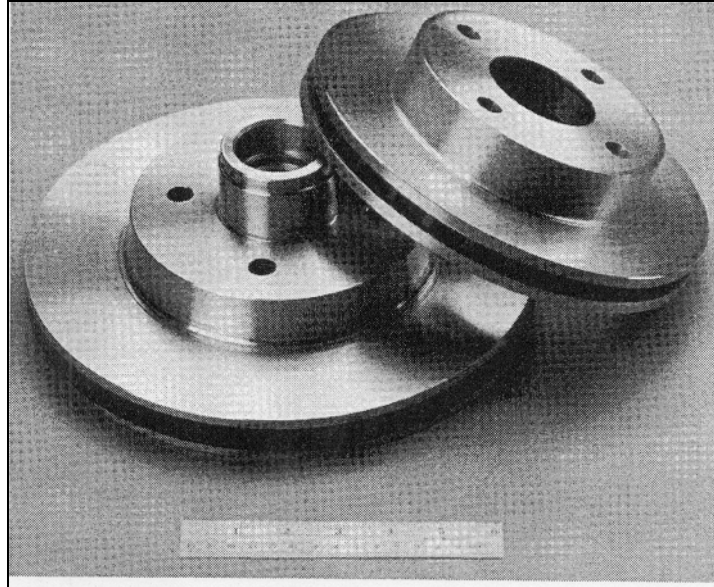
Figure M10.4.3.2.3.3 (b) Photograph of a rotor brake disc, made from Duralcan ® cast Al-10wt%Si / 20vol% SiC.
