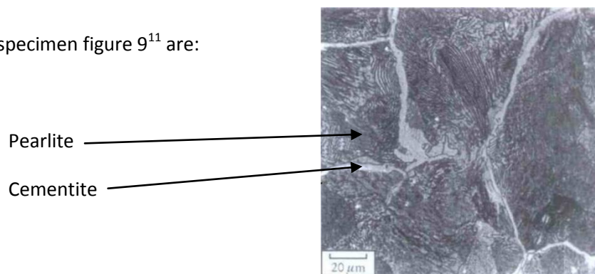
Figure 9: A hypereutectoid steel carbon
